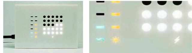
Figure 1. Local Energy Indicator. Current levels of wind and solar power from domestic solar panels and wind turbine are displayed, as well as the total amount of stored energy available.
